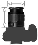
Flat ports are recommended for macro and telephoto lenses. Note that if a port is long enough to accommodate the full length of a 1:1 macro lens, the lens may vignette at infinity behind a flat port.
