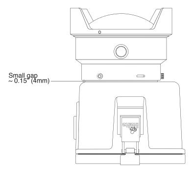
7. Tighten all three thumbscrews while holding the port firmly towards the housing. The thumbscrews should thread in completely until the head touches the port. If the screws are difficult to turn and/or they bottom out before their heads are flush, it is an indication that the port is not pushed far enough down on the housing.
