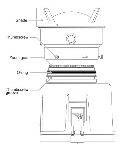
6. Press the port firmly towards the housing until the base of the port is almost flush with the housing front. If there is resistance, remove the port and re-check that the thumbscrews are loosened and the o-ring is properly lubricated.
