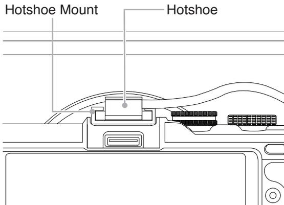
3. Push the Hotshoe forward until it is unable to go any farther. The Hotshoe must be pushed all the way forward to make proper contact with the camera and provide TTL operation. Make sure the Hotshoe wire does not interfere with any housing control operations.
