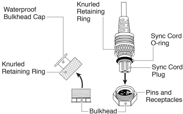
4. Rotate the Knurled Retaining Ring until snug on the housing bulkhead. Do not use pliers or tools to tighten the retaining ring.
