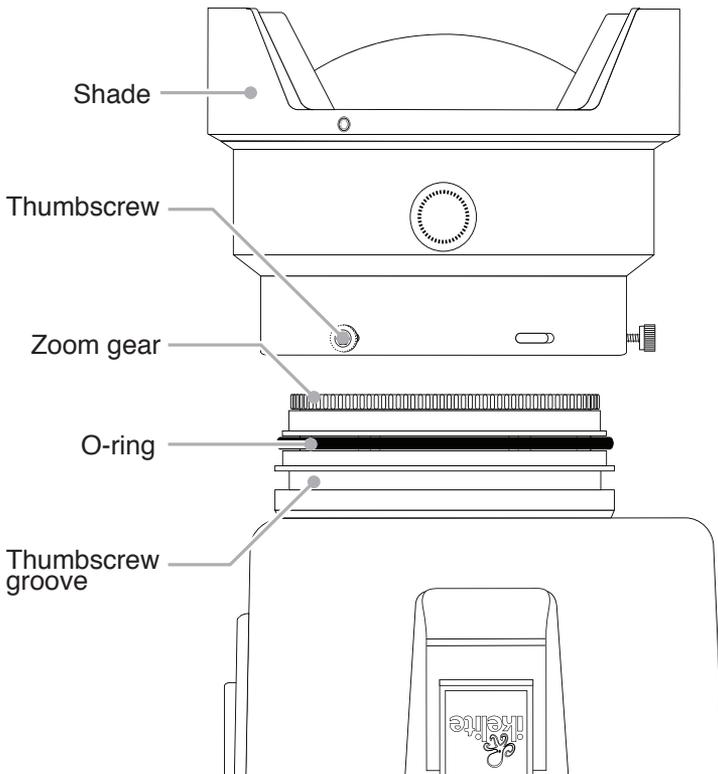
6. Press the port firmly towards the housing until the base of the port is almost flush with the housing front. If there is resistance, remove the port and re-check that the thumbscrews are loosened and the o-ring is properly lubricated.
