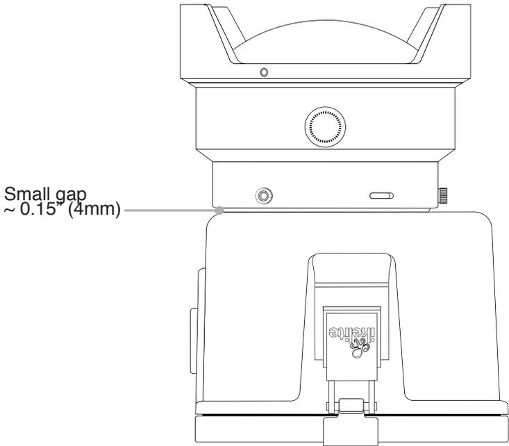
7. Tighten all three thumbscrews while holding the port firmly towards the housing. The thumbscrews should thread in completely until the head touches the port. If the screws are difficult to turn and/or they bottom out before their heads are flush, it is an indication that the port is not pushed far enough down on the housing.
