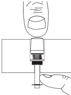
3. Press and release the push button several times to work the lubricant into the o-ring.
