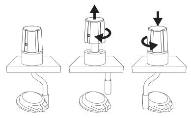
» If the control knob stops and the desired effect hasn't occurred, repeat step 2 to reverse directions.
