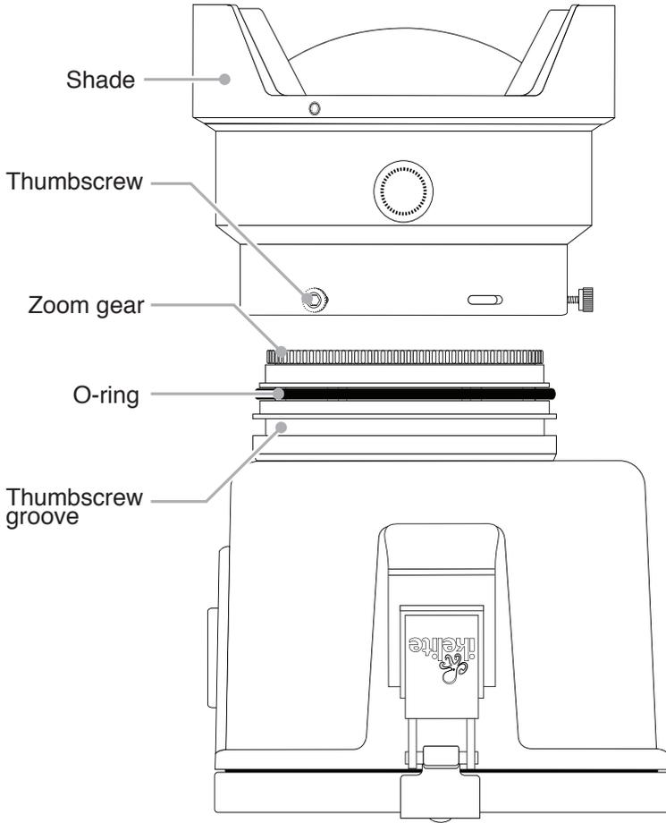
6. Press the port firmly towards the housing until the base of the port is almost flush with the housing front. If there is resistance, remove the port and re-check that the thumbscrews are loosened and the o-ring is properly lubricated.
