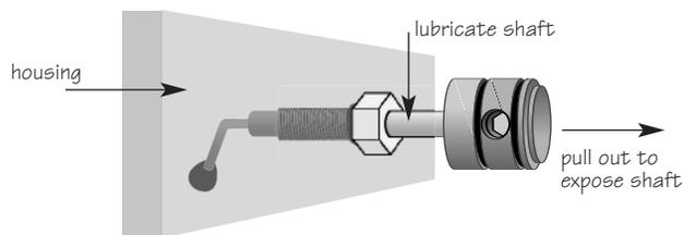
pulled out, exposing the shaft (see drawing).
