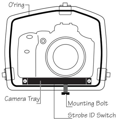
**NOTE:** Strobe ID Switch located on bottom of camera tray.
