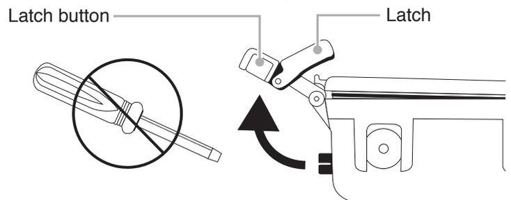
2. The back of the housing will be compressed by pressure underwater or after air travel. Rotate the latch fully to break the seal of the housing. Do not use metal objects or tools to pry the back open.
