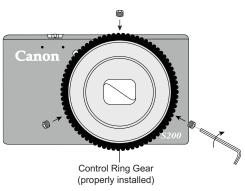
head wrench as show in the Diagram. **Do not** overtighten or you will damage the gear. Make sure to test it's function once installed.
