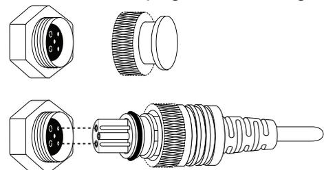
4. Hand-tighten the retaining ring.
