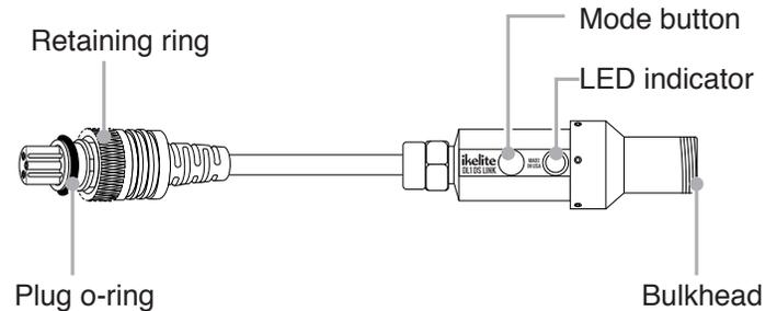
2. Apply a very thin, even layer of lubricant on all threads, sealing surfaces, and the exposed portion of the plug o-ring. Do not allow lubricant to get into the pins and receptacles of the plug or bulkheads.
