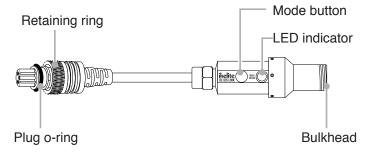
2. Apply a very thin, even layer of lubricant on all threads, sealing surfaces, and the exposed portion of the plug o-ring. Do not allow lubricant to get into the pins and receptacles of the plug or bulkheads.
