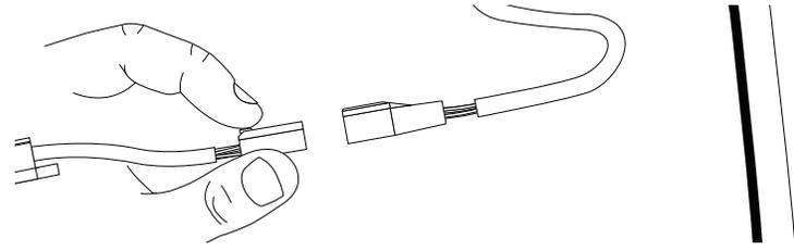
2. Align TTL hotshoe and bulkhead connector ends and push together until tab clicks into place.
