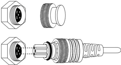
4. Hand-tighten the retaining ring.
