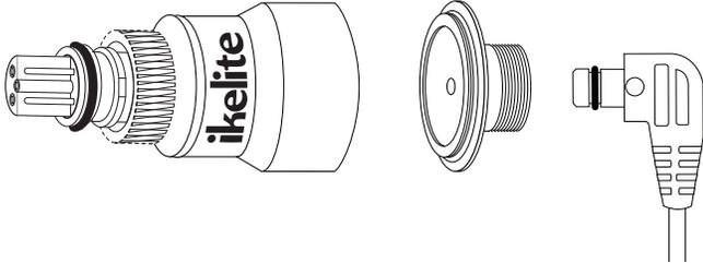
2. Attach a compatible fiber optic cord to the fiber optic port.
