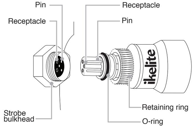
5. Align plug and insert into the strobe bulkhead. Each male pin mates with a female receptacle. Failing to line up the contacts properly before tightening may result in damage to the converter and/or strobe.
