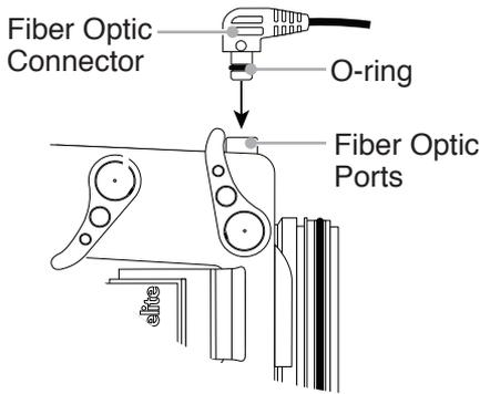
2. Ensure that the fiber optic cord o-ring is in place. This o-ring does not provide waterproofing, however it does keep the fiber optic cord in place.
