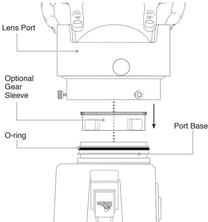
3. If using an optional Gear Sleeve, place it in the Port Base with the teeth side facing away from the housing.
