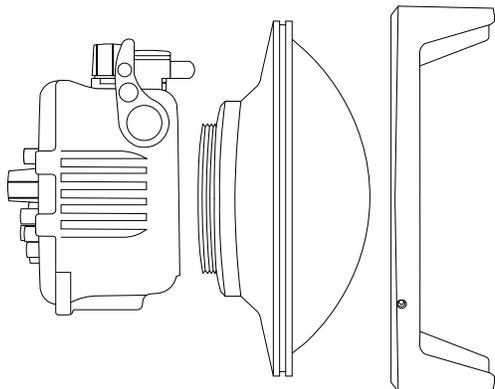
6. Facing the front of the housing, rotate the Dome Port clockwise and tighten until snug.
