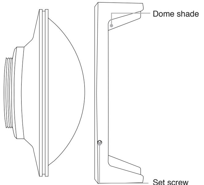
3. Check that the o-ring is in its groove on the back of the dome port.
