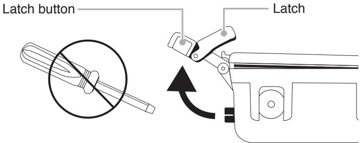
2. The back of the housing will be compressed by pressure underwater or after air travel. Rotate the latch fully to break the seal of the housing. Do not use metal objects or tools to pry the back open.
