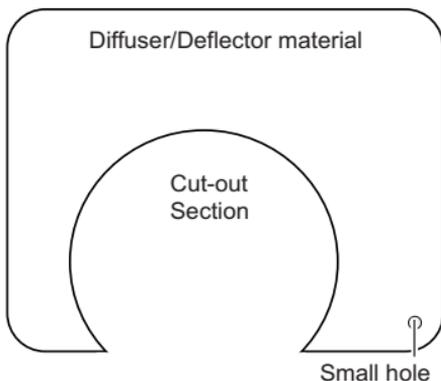
Note the Small Hole. To avoid losing the Diffuser or Deflector, you can attach a fishing line or string to this hole.
