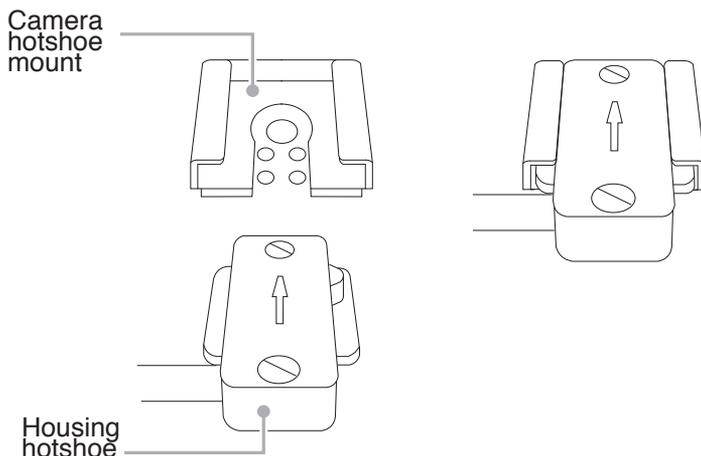
2. Slide the housing hotshoe into camera's hotshoe mount until it stops.
