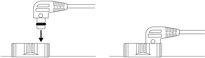
4. Attach the other end of the fiber optic cord to a compatible strobe.
