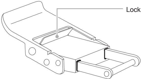
2. Lid snaps are designed to provide enough force to compress the o-ring for a proper seal. Keep firm pressure against the lid snap while lifting it away.
