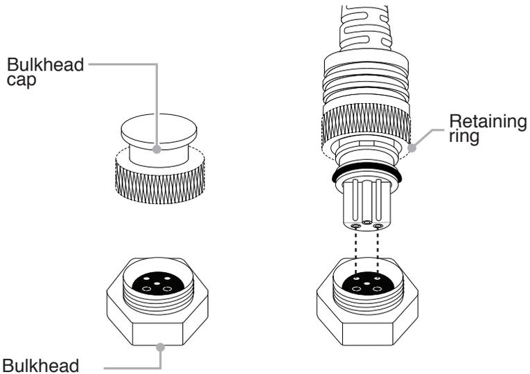
3. Align plug and insert into the housing bulkhead. Each male pin mates with a female receptacle. Failing to line up the contacts properly before tightening may result in damage to the converter plug and/or housing bulkhead.
