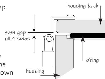
**Double check** - Once the housing is closed, check the o'ring seal. Check the gap between the housing back and the housing, it should be even all the way around.
