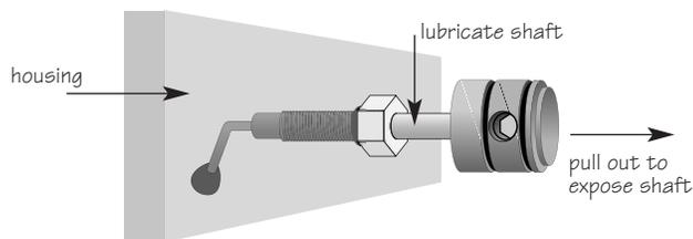
2. Some of the controls have long shafts. These controls can be pulled out, exposing the shaft (see drawing). To lubricate the control, gently pull on the knob until the stainless steel shaft is exposed. Lightly lubricate the shaft, then move the shaft in and out several times. This will lubricate the x'ring in the Ikelite control gland. This should be done before using the housing after a prolonged storage period, or once a week when the housing is in use.
