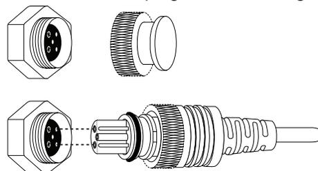
4. Hand-tighten the retaining ring.
