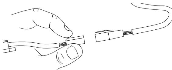
2. Align TTL hotshoe and bulkhead connector ends and push together until tab clicks into place.
