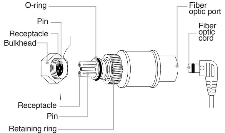
5. Align plug and insert into the strobe bulkhead. Each male pin mates with a female receptacle. Failing to line up the contacts properly before tightening may result in damage to the converter and/or strobe.
