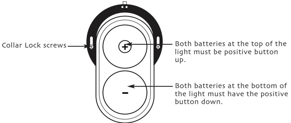
**COLLAR:** The two screws that secure the Collar Lock should be as tight as possible while still allowing the Collar Lock to move freely.
